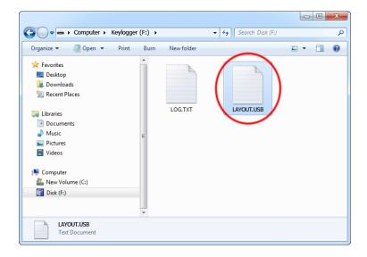
To enable the layout, safely remove the flash disk. On power-up, the layout file will be loaded automatically.
