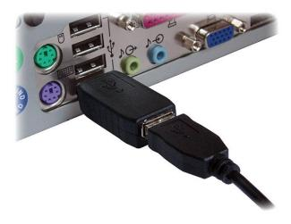
**To view recorded data**, plug the device in-between the keyboard and USB port, and press the 3-key combination **simultaneously** (by default K, B, S)
