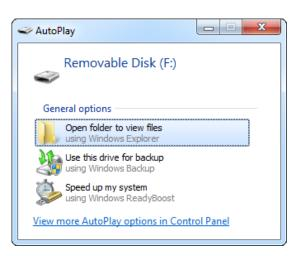
Depending on the drive letters available, the device will be visible as a new drive, for example F:. Use the systems file manager to browse this disk (for example *Explorer*). The keyboard will be disconnected and unavailable, so the mouse must be used to browse the disk.
