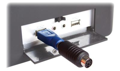
After a few seconds, the hardware keylogger will automatically get detected as a mass storage device. The operating system will use the standard built-in mass storage driver (*MS Windows 7* in the following examples).
