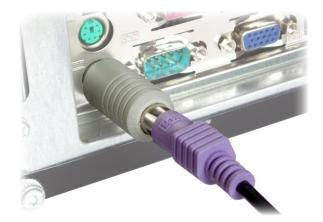
**To view recorded data**, plug the device in-between the keyboard and PS/2 port, and open a text editor (such as *Notepad*). Then press the 3-key combination **simultaneously** (by default K, B, D)
