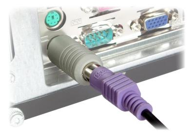
Connect the *KeyGrabber PS*/2 between the keyboard and the PS/2 port. Keystroke logging will start automatically on power-up.
