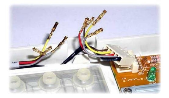
Finally, assemble the black 0.1" connectors, inserting the sockets into the casing. **The connector pinout must match the module pinout on both sides**, as shown on the picture below.
